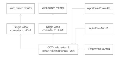
A proportional joystick provides a simple and convenient way to add X-Y control (zoom-focus) to a zoom camera.
